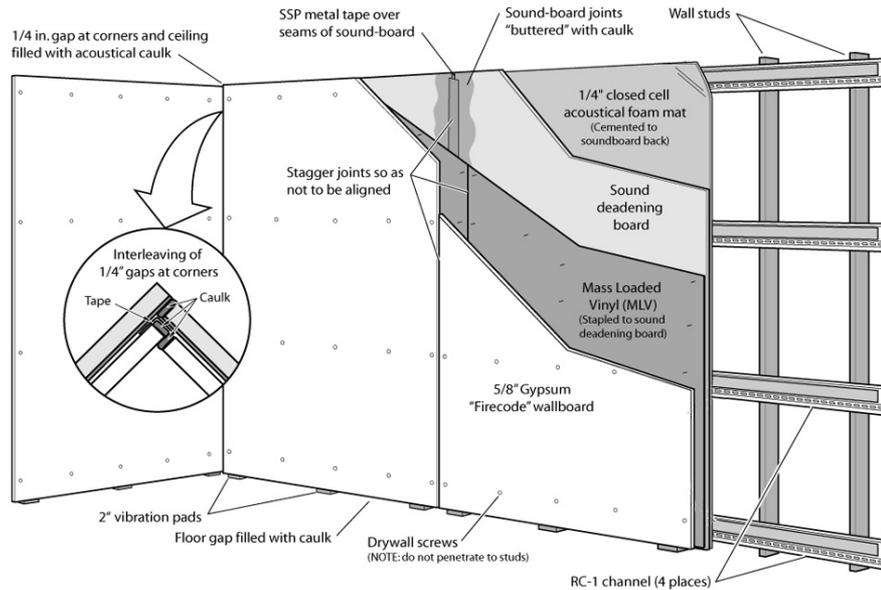
**When your job asks for two layers of board, you should offset your seams for every layer. This ensures sound transmissions are blocked throughout the wall assembly.**
